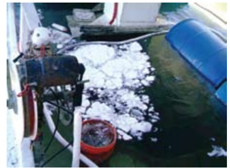
A C.I.Agent® QDB placed around the engine compartment and one pound of C.I.Agent® Granules dispersed inside the boom to solidify the motor oil.
