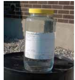
Water sample from the EVAC Filter was lab tested and showed "non detect" for hydrocarbons.
